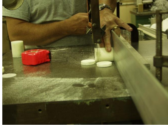
Figure 4. Specimen length manufacturing
