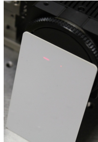
Etalon beamsplitter (left), ten signal beams and reference beam focused on the detector (right)
