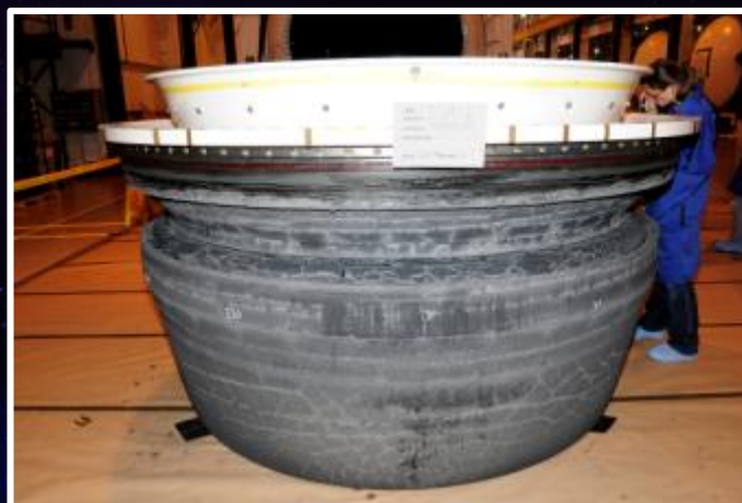
DM-1 Nozzle post-fire inspection
