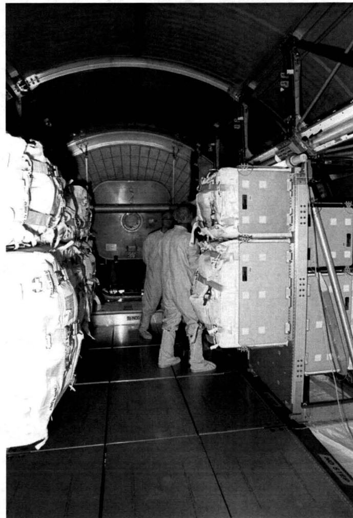
KSC-01PP-0726: Workers in the Space Station Processing Facility are removing contents from the Multi-Purpose Logistics Module (MPLM) Leonardo to begin removing the contents after STS-102. The MPLM brought back nearly a ton of trash and excess equipment from the Space Station. 6
