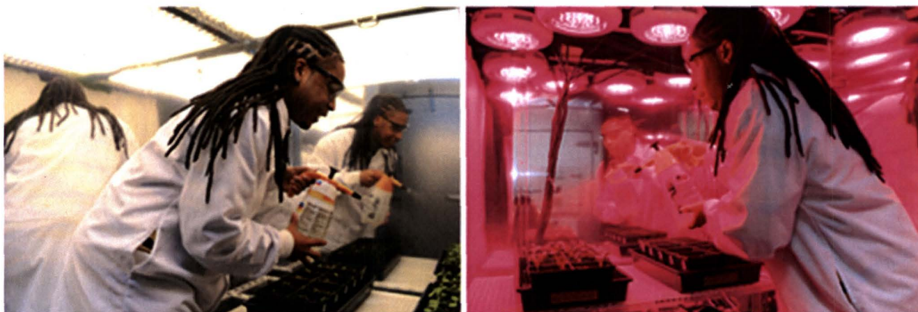
Figure 1. Kennedy Space Center Environmental Growth Chambers with UFO Red and Blue LED treatment (right) and daylight fluorescent tubes treatment (left).
