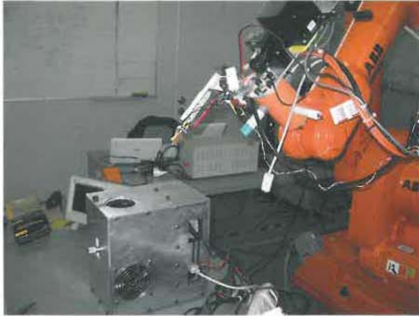
Figure 2: Mechanical positioning used in source characterization. The golden horn is the receiver, being positioned by ABB IRB1600. In this picture, \phi = 180 deg, \theta = -40 deg. To reduce reflexions from the robot, a square sheet of ECCOSORB was placed right behind the feed horn, which is not shown in this picture. Here the robot is sampling the E-plane of the source.
