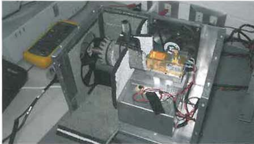
Figure 1: Microwave source interior setup. The feed shown in the figure was later replaced by an open waveguide with circular flange. The feed and surroundings are all covered with ECCOSORB to reduce reflexions. The fan was used to control temperature in case of overheating.
