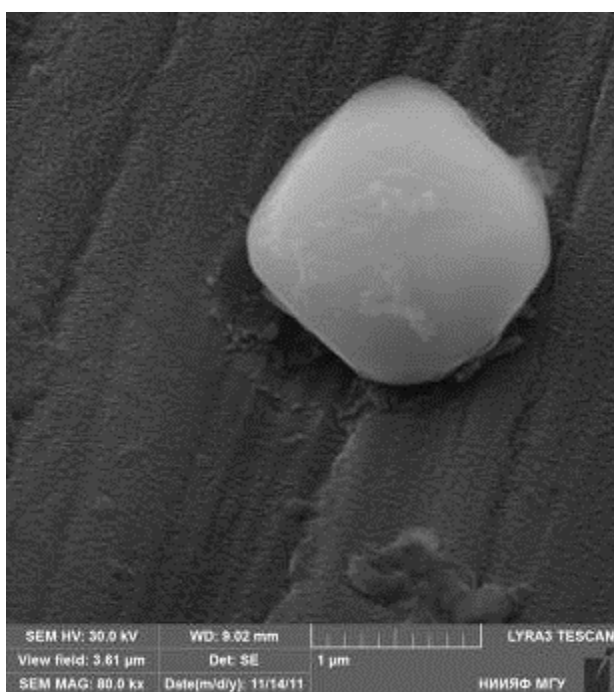
Fig. 12 Low Velocity CrO x Microparticle on Surface of Titanium Sample
