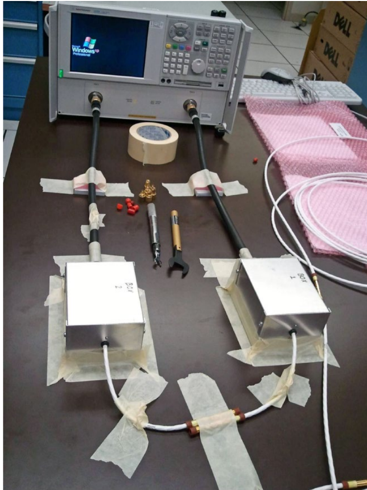
Figure 4.—Typical calibration of performance network analyzer (PNA) with baluns and pigtail cables terminated with the calibration kit.
