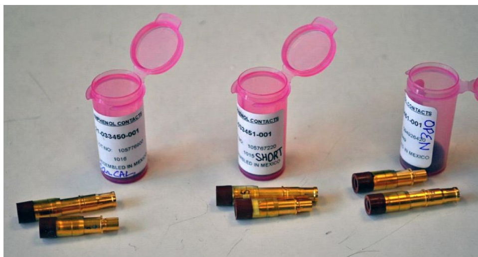
Figure 5.—Load, short, and open terminators for the 150-Ω performance network analyzer (PNA) calibration kit.
