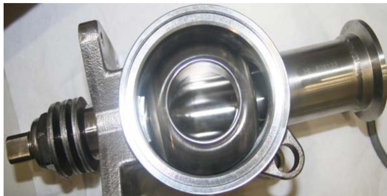
Figure 23 Disassembled Valves Appeared Shiny and Clean
