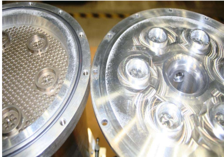
Figure 22 Top (13X) Cover and Baffle Plate Assy Showed a Small Amount of Fine Dust Passed Thru 50 \mu\text{m} Screen
