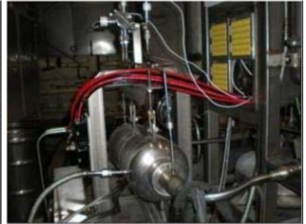
Power Cable path to core
