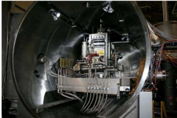
FPS-PTC Stirling & 7 Pin Rx Core Sim Testing
