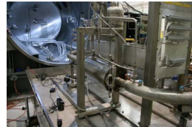
Full-scale NaK Pump Test
