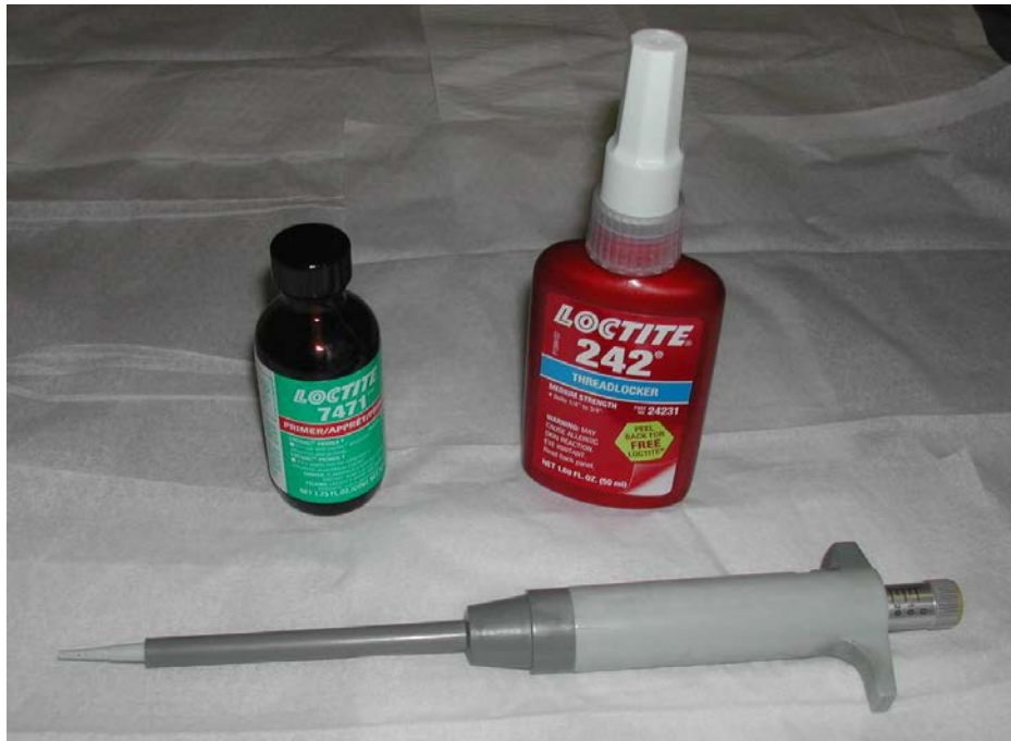
FIGURE 22 - LOCTITE 242, PRIMER T, AND MICROPIPETTE
