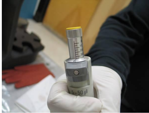
FIGURE 2 - MICROPIPETTE WITH GRADUATIONS TO CONTROL AMOUNT OF LOCTITE
