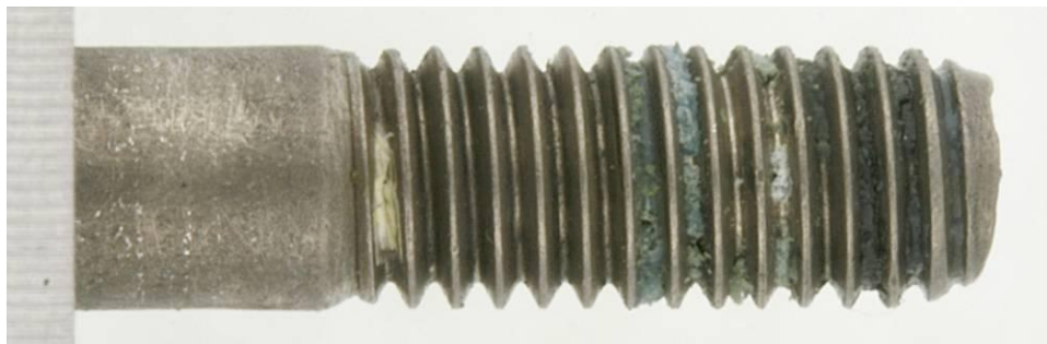
FIGURE 26 - 25 \mu L ON NUT THREADS ONLY
