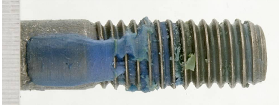
FIGURE 27 - 35 \mu L ON BOLT THREADS AND 25 \mu L ON NUT THREADS
