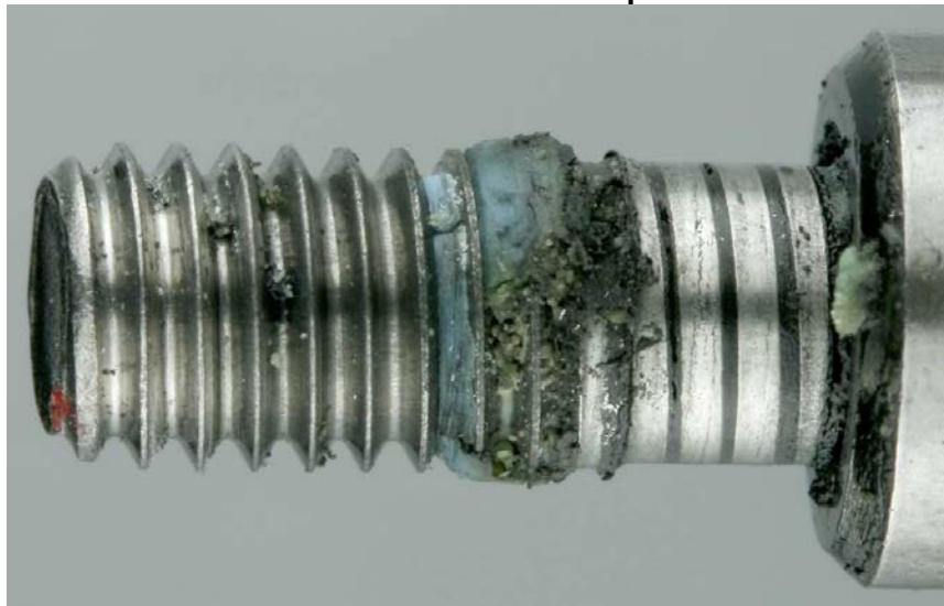
FIGURE 32 - AFTER VIBRATION TEST - 35 \mu L ON BOLT THREADS
