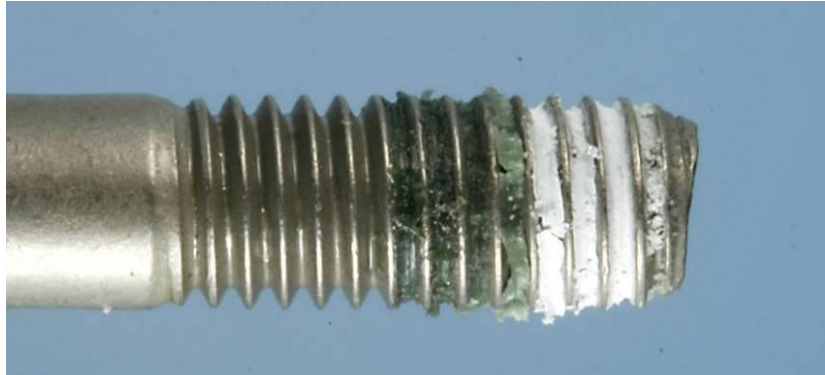
FIGURE 20 - LOCTITE 290 IN OPEN INSERT
