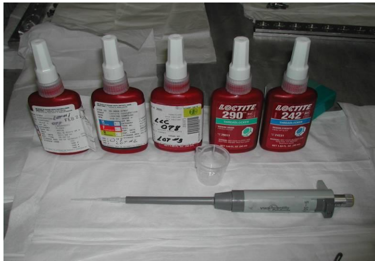
FIGURE 1 - MICROPIPETTE WITH DISPOSABLE TIPS AND TARE CUP
