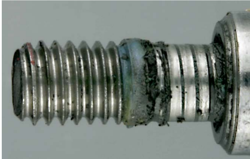
FIGURE 31 - AFTER VIBRATION TEST - 20 \mu L ON BOLT THREADS
