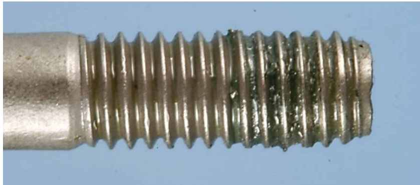
FIGURE 19 - LOCTITE 290 IN BLIND INSERT
