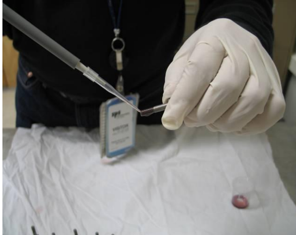
FIGURE 4 - LOCTITE APPLIED TO BOLT THREADS
