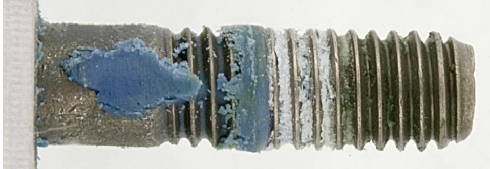
FIGURE 25 - 35 \mu L LOCTITE 242 ON BOLT THREADS ONLY
