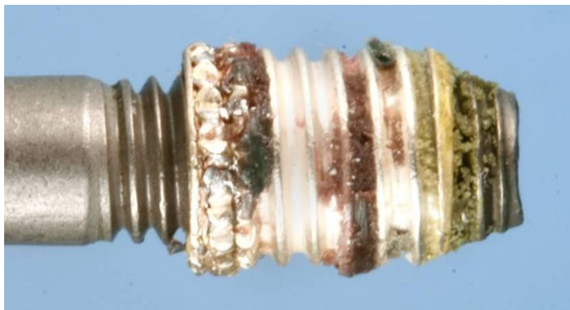
FIGURE 21 - LOCTITE 290 WITH INSERT PULLED OUT
