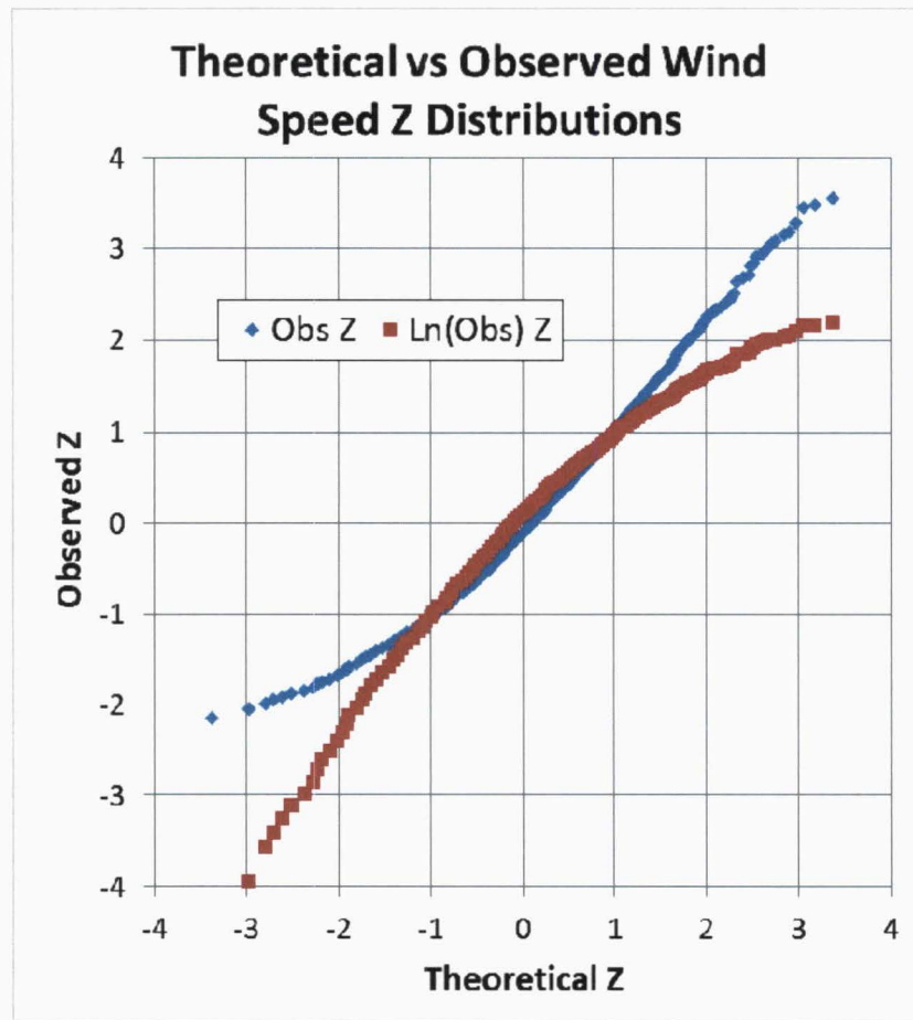
Figure 3. Curves showing the relationship of the z values for the observations (blue) and the ln of the observations (red) to the theoretical Gaussian z values.
