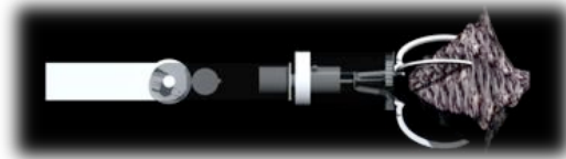
Figure 5. GeoLab sample manipulator (CAD model).
