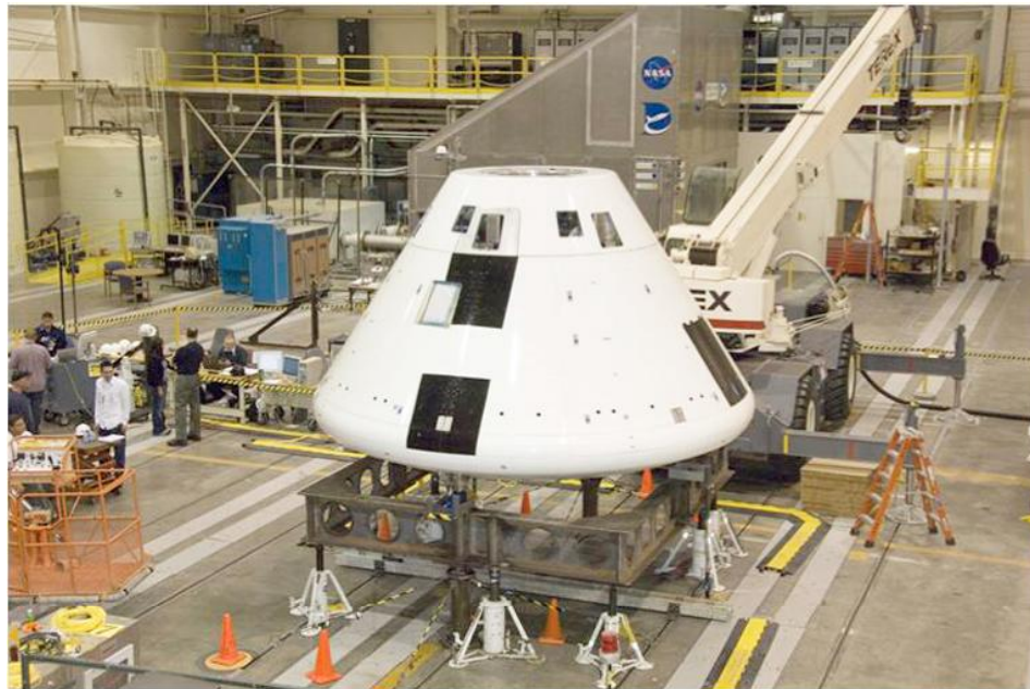
Figure 8. Iyy/Izz test setup in the Flight Loads Lab at NASA Dryden.
