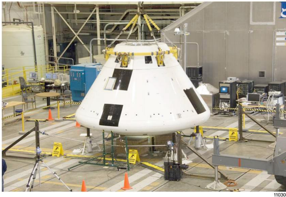
Figure 6. Torsion pendulum test setup at the Flight Loads Lab at NASA Dryden.
