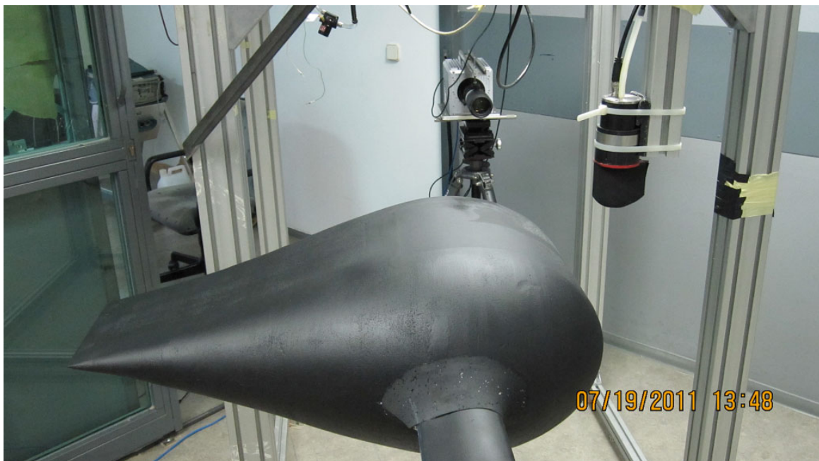
Figure 3.—Close-up picture of airfoil (DBKUP 003, chord = 0.710 m), TSI droplet generator and the high speed camera.
