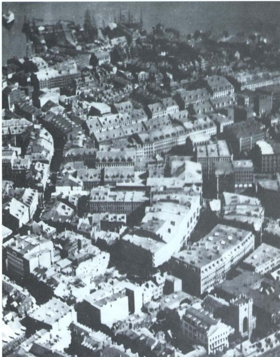
Figure 3-5 A portion of an aerial photograph of downtown Boston, MA, obtained by aeronauts James W. Black and Samuel A. King from a tethered balloon at an altitude of 1,200 ft on October 13, 1860. It is believed to be the first aerial photograph taken from a captive balloon in the United States and the earliest aerial photograph still in existence. It was obtained using a wet collodion plate (used with permission of the Smithsonian Institution, Washington, DC; #3B-15472).
