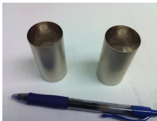
Fig. 1: Pure nickel mirrors electroformed using pulse plating technique
