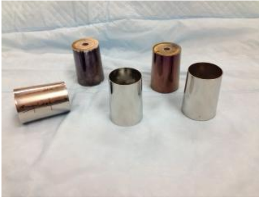
Fig. 2: Two conical mandrels used for replication tests (shown in background); three un-coated conical shells, replicated from these (foreground).
