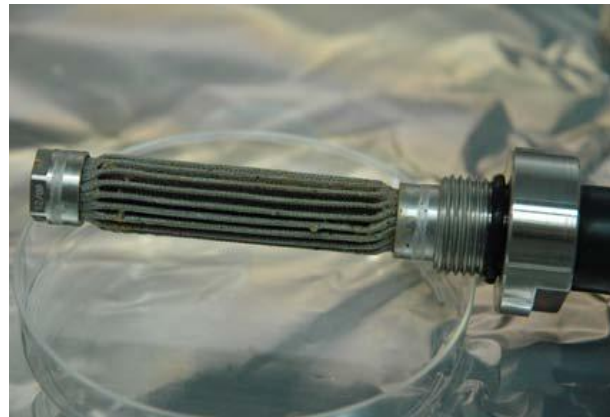
Figure 2. Mesh filter after removal from the housing.
