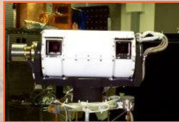
Mars Phoenix Surface Stereo Imager (SSI) (Image Courtesy of Univ. of Arizona)
