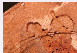
Micrographs of copper electrode and copper flakes recovered from electrode.
