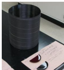
Wound and cured IL epoxy/carbon composite
