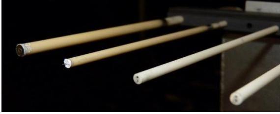
Figure 6. Probe array with Faraday probe at far left.
