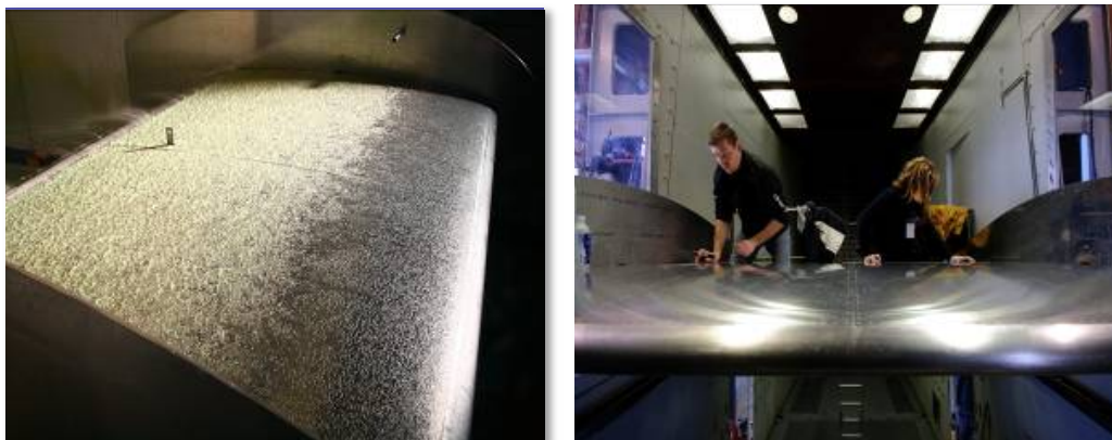
Figure 6.—Photographs of thin, high-performance wing model installed in the NRC PIWT facility.
