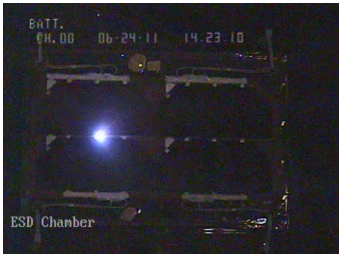
Fig. 12. Image of arc flash on Coupon A string 1.
