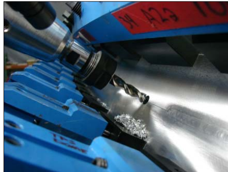
Start hole for self-reacting FSW
