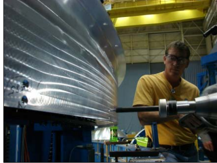
RWT drilling tooling attachment holes
