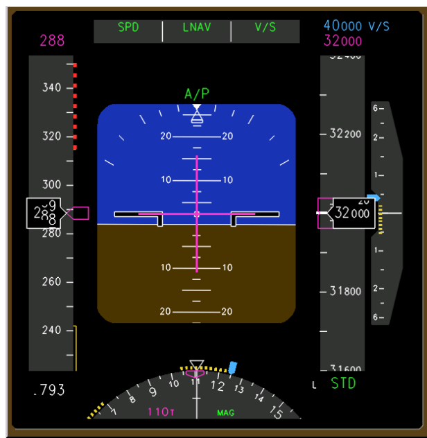
Figure 5. Displays of Track/Heading and Vertical Speed MR Bands on PFD
