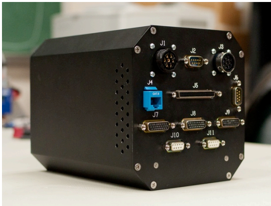
Figure 5: Avionics for Subscale Remotely Operated Vehicles (ASROV) flight computer
