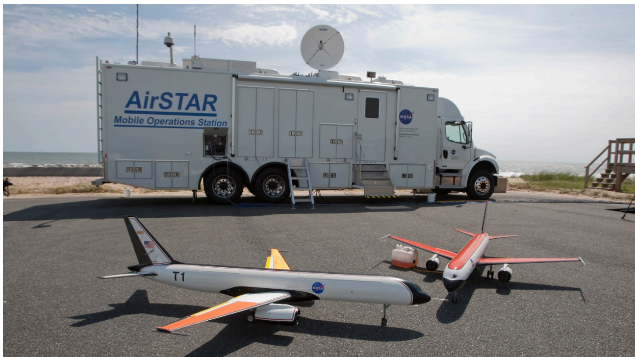
Figure 1 Mobile Operations Station (MOS) at the NASA Wallops Flight Facility UAV runway with two 5.5% dynamically scaled vehicles (tail numbers T1 and T2) in the foreground.
