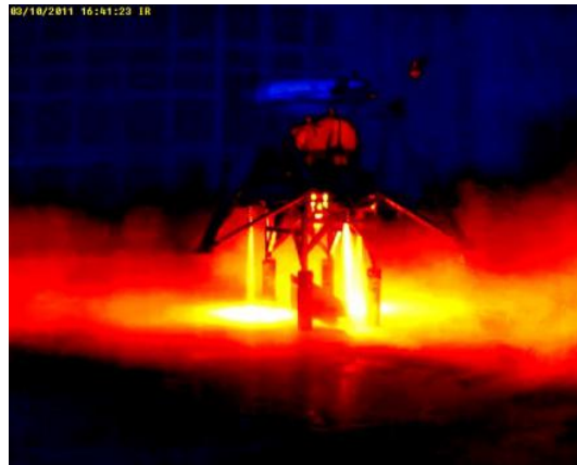
Figure 5: Infrared view of WGTA strap-down hot fire test
