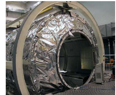
External Passive Thermal Control
