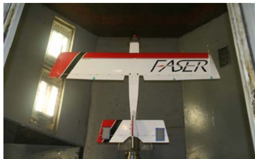
Figure 1. FASER mounted in the NASA LaRC 12-FT Low-Speed Tunnel.
