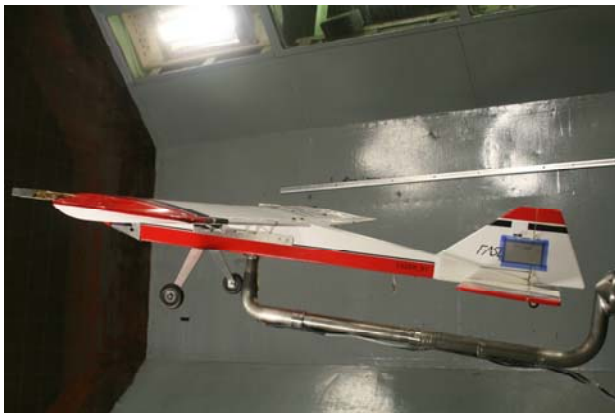
Figure 3. FASER mounted for roll oscillation runs.
