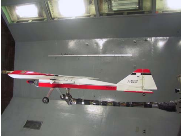
Figure 2. FASER mounted for static force and moment tests prior to the current forced oscillation.
