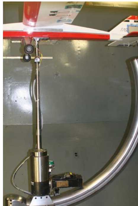
Figure 4. FASER mounted for yaw oscillation runs with the wings parallel to the test section floor.
