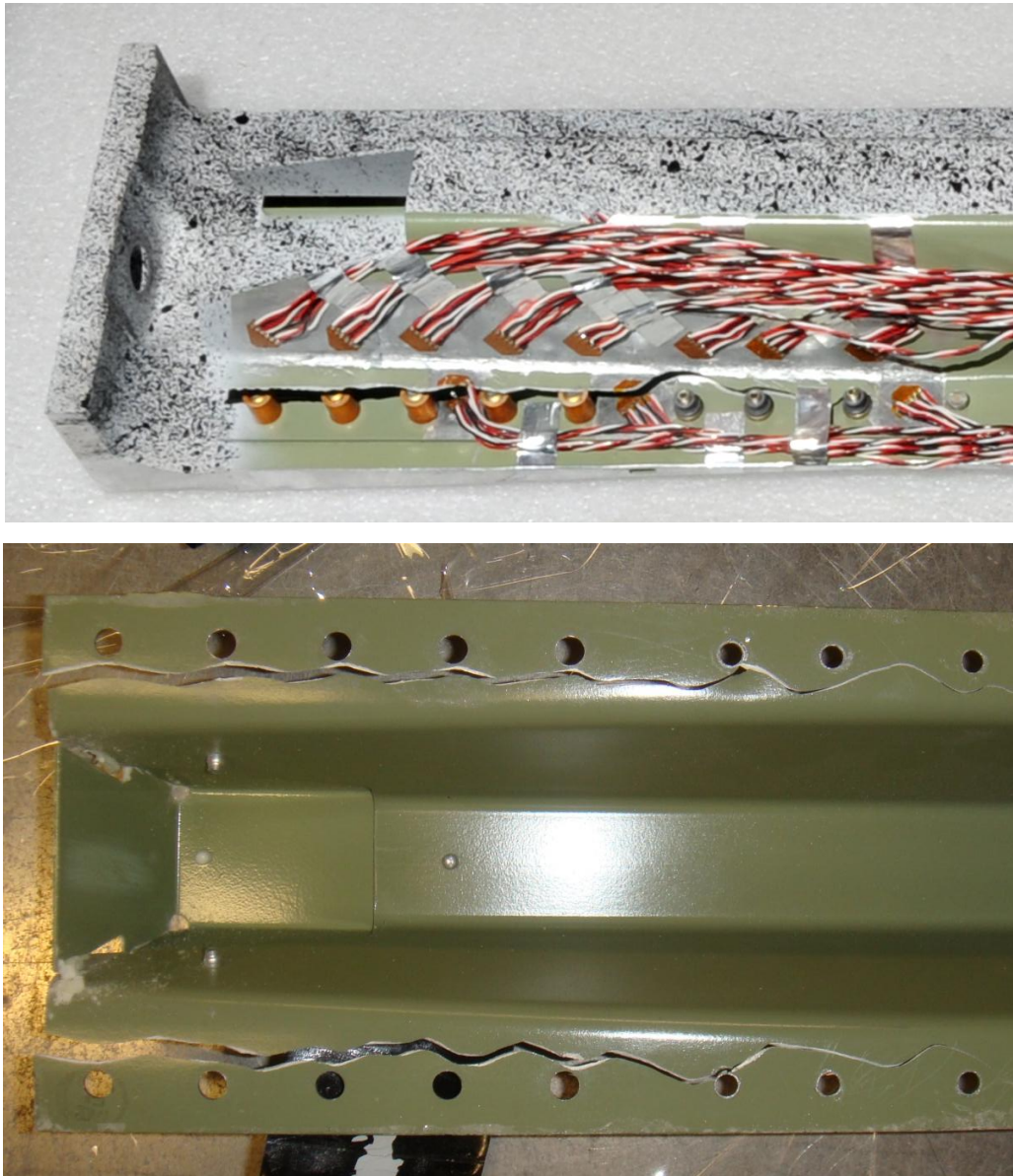
Figure 23. Similarity of failure between cracked stringer removed from ET-137 (bottom) and stringer bending test article after failure (top).
