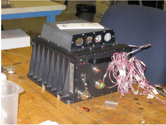
Heavy Box Approximately 50 Lb First Predicted Significant Mode is at 847 Hz
