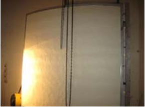
Orthogrid Panel with TPS Installed - View From Reverberant Chamber
