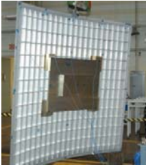
Orthogrid Panel With An Avionics Panel Simulator
