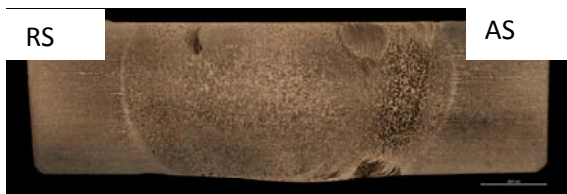
Figure 6. Transverse view of H-TSW nugget taken near the end of the 210cm long weld panel.
