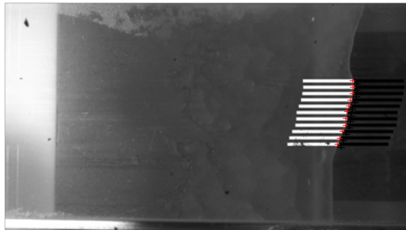
Figure 8.—An example frame from a multiple ROI analysis used for cases where the ice-growth was not uniform across the airfoil or for cases where ice or water contamination affected the analysis.
