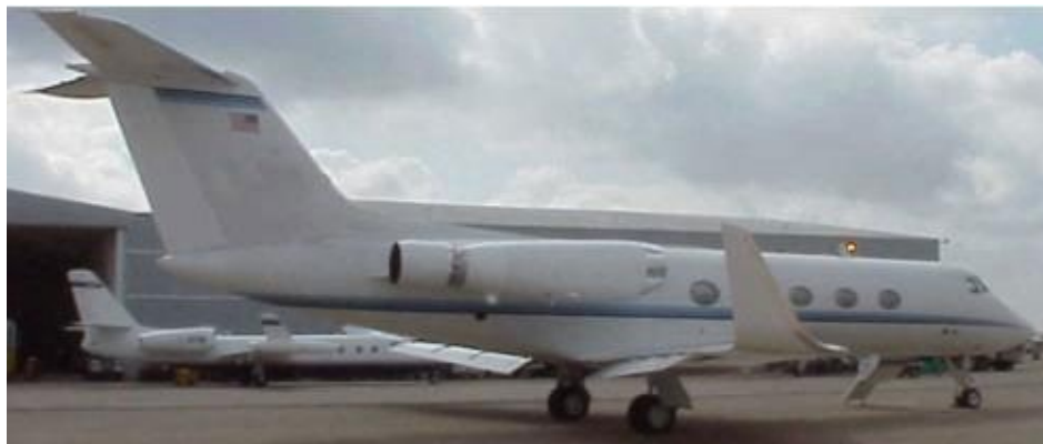
Figure 1.—Alternating lobe mixer-ejector concept (ALMEC) suppressor system installed on a Gulfstream G-II aircraft (Ref. 4).
