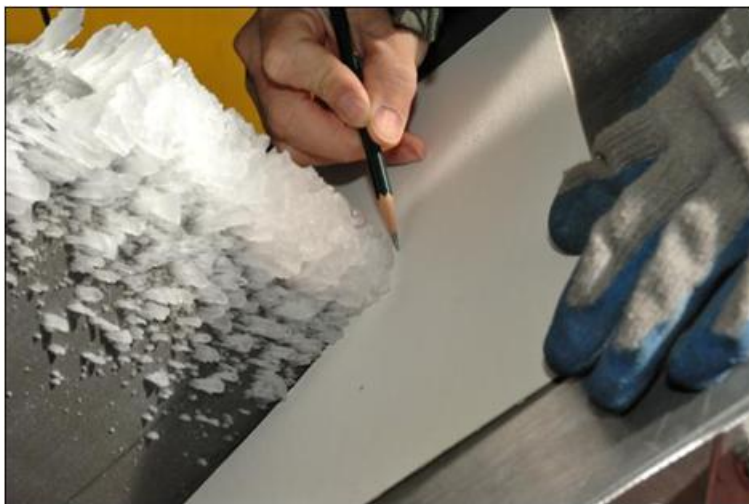
Figure 1.—Cross-sectional ice shape tracing method.
