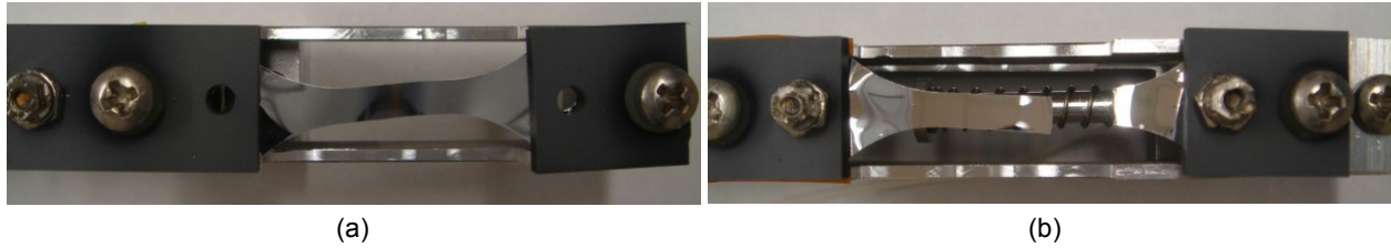
Figure 9.—(a) Unstressed VDA/CP1 sample AO-U-7 flown on the ram facing side of MISSE 6. (b) Stressed VDA/CP1 sample AO-S-5 flown on the ram facing side of MISSE 6. Sample broke sometime during the exposure on ISS.
