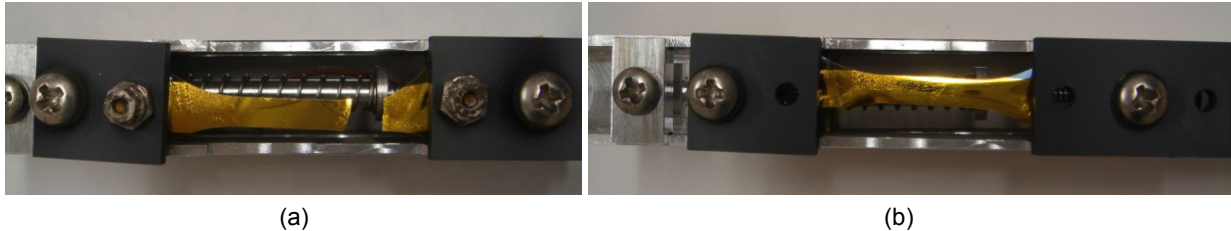
Figure 6.—(a) SiO x /Kapton HN stressed sample AO-S-6 from ram side tray G3 showing break. (b) SiO x /Kapton HN stressed sample UV-S-8 from wake side tray 62 showing coating cracking.
