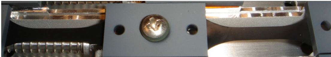
Figure 14.—Stressed (left) and unstressed (right) black Kapton XC flown on the wake side of MISSE 6
