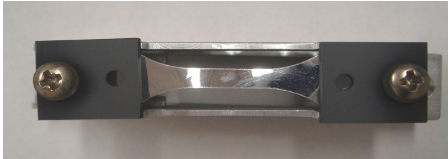
Figure 10.—FEP/VDA exposed on MISSE 6 ram side in unstressed condition (AO-U-8).
