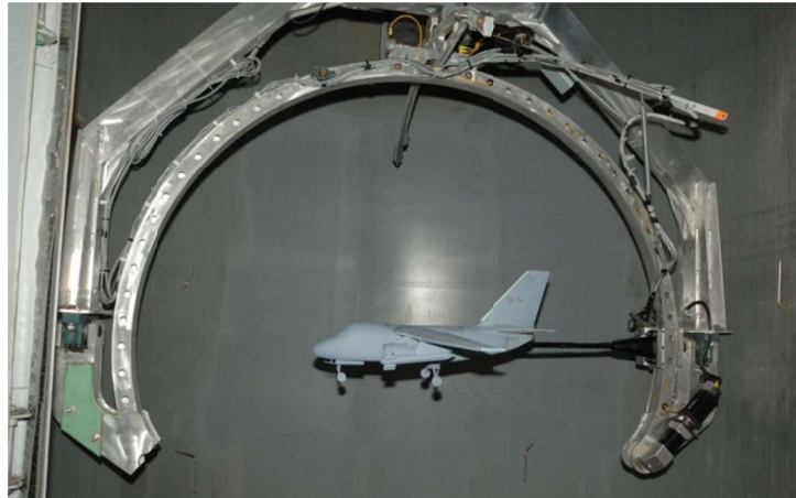
Figure 1.—S-3B Viking model in LAMP test section.
