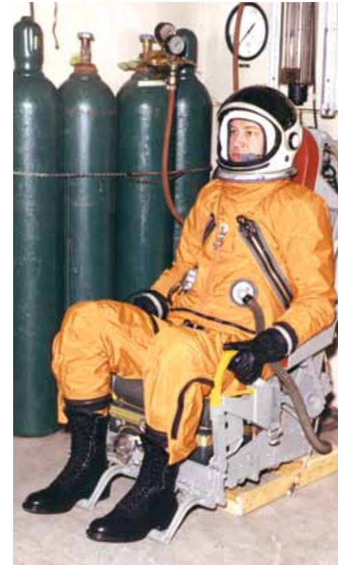
The A/P22S-2 air inlet and suit controller was on the right side of the suit and the air exhaust was on the left. Note the diagonal zippers for the U-shaped entry. Joe Ruseckas is wearing the suit while sitting in an ejection seat used for fittings.
