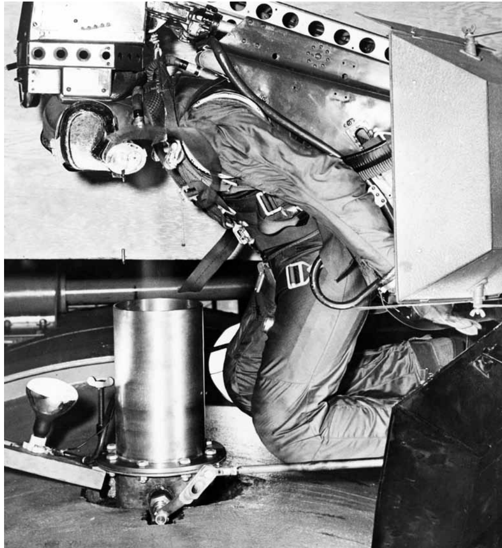
One of the more unusual tests conducted on pressure suits was this visor windblast evaluation. The pilot, strapped into an ejection seat, was suspended over an icing chamber that blasted high-velocity air at the visor. Note the frost on the goggles. Similar tests were run with warm air.
