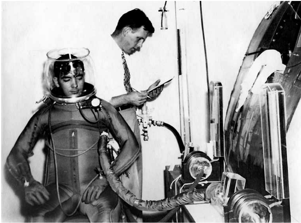
John Flagg wears the Model 2 suit seated next to the F4U cockpit (extreme right) in Worcester with Ken Penrod in the background. For this suit, David Clark Company eliminated the lace adjustments and tailored the suits for each individual. Note the zippers coming down from the shoulders into the arms, across the upper chest, and vertically down to the crotch. Initial attempts at finding an effective manner to don and doff a pressure suit were elusive.
