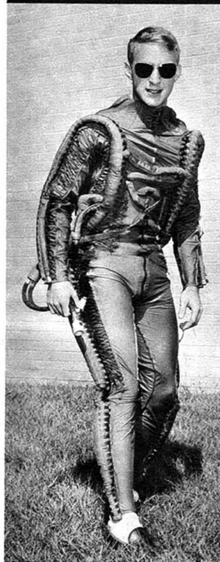
Above: David Clark Company S612 partial-pressure suit gloves were typical of the gloves used with later pressure suits. The gloves had leather palms and nylon backs. These particular gloves have the pressure lead on the pinky side; the MC-3 and MC-4 suit had pressure leads on the thumb side. Note the lace adjustments on the back.
