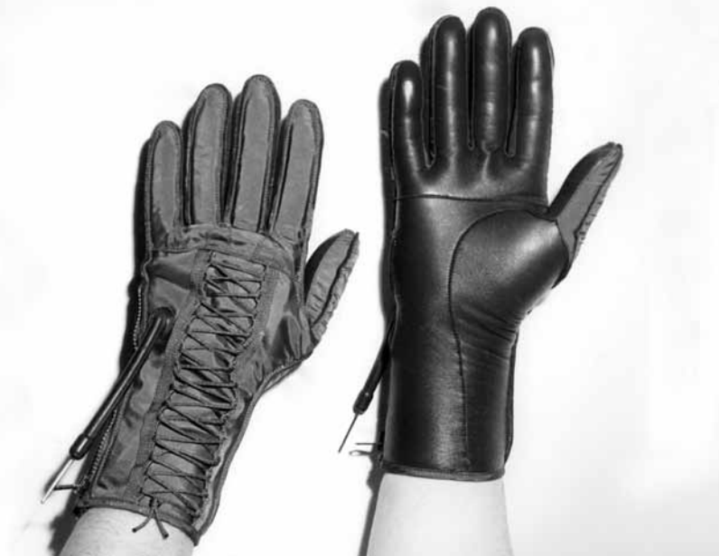
Above: David Clark Company S612 partial-pressure suit gloves were typical of the gloves used with later pressure suits. The gloves had leather palms and nylon backs. These particular gloves have the pressure lead on the pinky side; the MC-3 and MC-4 suit had pressure leads on the thumb side. Note the lace adjustments on the back.
