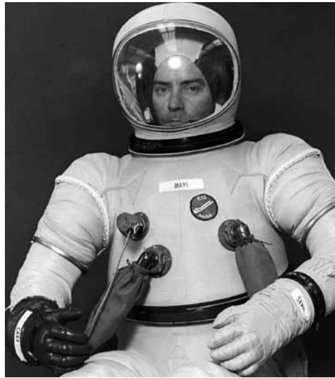
The ILC Dover Emergency Intravehicular Suit (EIS) operated at 8 psi to support reasonably rapid decompression from a 14.7-psi cabin pressure without risk of decompression sickness. The entire suit, except for the waist disconnect ring, was fabricated of flexible materials, including the helmet and face shield.
