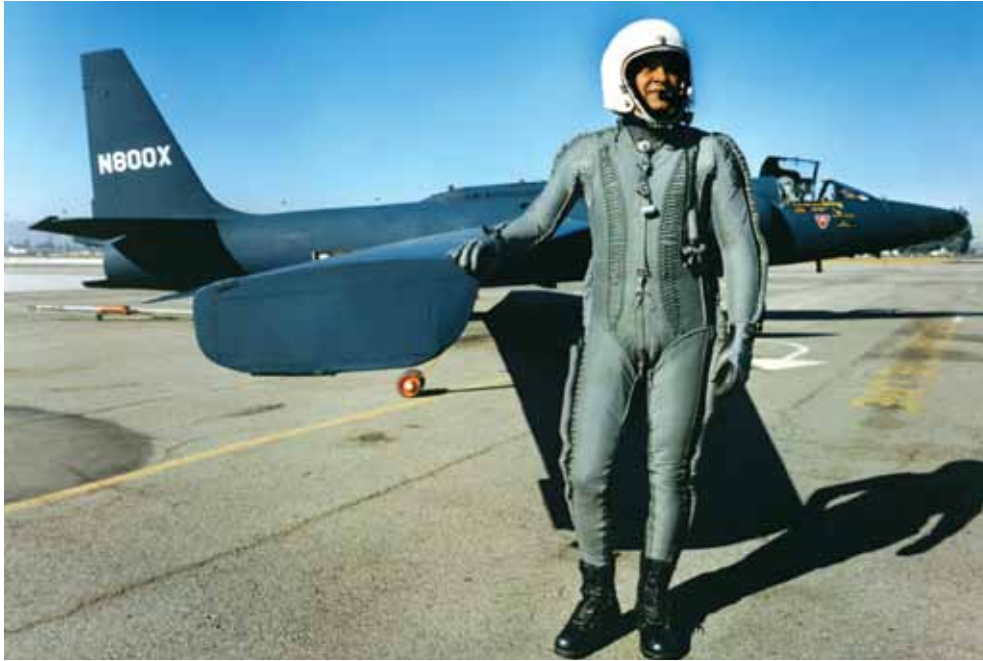
Francis Gary Powers wearing an MC-3 partial-pressure suit and MC-2 helmet in front of a Lockheed U-2A. The MC-3 had additional lacing, extending up the inner thigh, the small of the back, and down the chest, to provide better control of the torso bladder and more variation in circumferential fit. Powers was shot down over the Soviet Union on May 1, 1960, and was not returned to the United States until February 10, 1962, in an exchange for Soviet KGB Colonel Vilyam Genrikhovich Fisher (aka Rudolf Abel), a Soviet colonel who was caught by the FBI.
