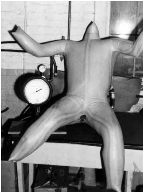
The first of the David Clark pressure suit for the U.S. Navy was this Experiment A. Obviously, this suit was never intended for anybody to wear—it was sewn closed at the neck, hands, and feet. The designers used this suit to determine a candidate fabric's reaction to pressure.
