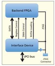
The **cPCI Interface** is a common interface between the cPCI bus and the backend FPGA. It is implemented as a separate interface device on the cPCI bus.
