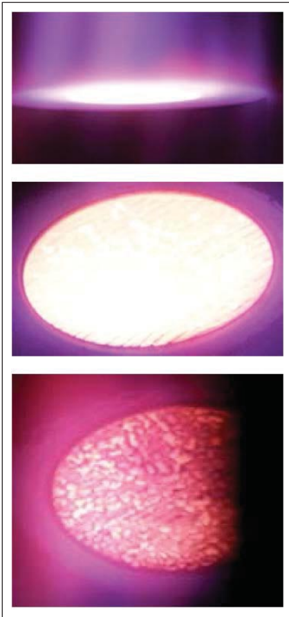
Figure 1. RICA Sample during plasma wind tunnel testing.
