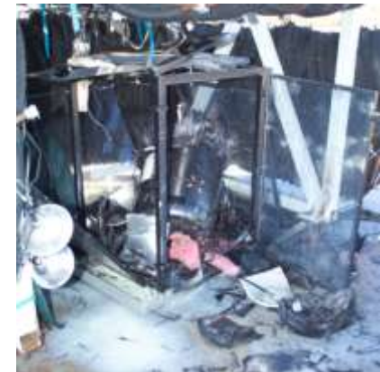
BBL rupture of a COPV
