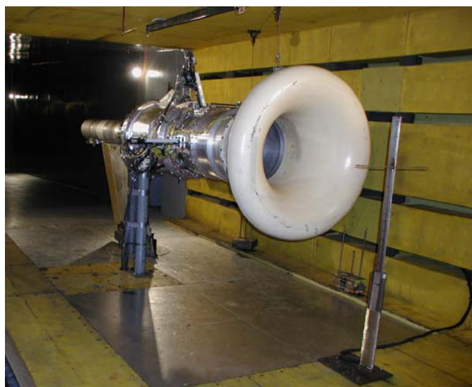
Figure 182. QHSF II Tunnel Installation, in Aerodynamic Performance Measurement Configuration.
