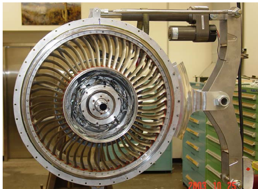
Figure 178. QHSF II Fan Stator and Rotating Stator Actuation Assembly on the NASA 22" Dummy Drive Rig.
