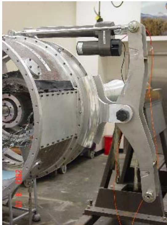
Figure 159. The Final Rotating Stator Actuation System Uses One Actuator and Horizontal Bar.
