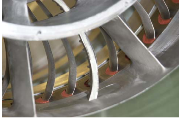
Figure 163. Aft Looking Forward View of Fan Frame and QHSF II Stator, With One Comb Rake Shown.
