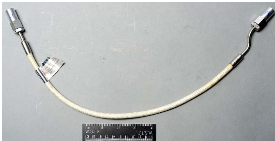
Fig. 2 Photograph of a Shuttle FCDC assembly (P/N 51009-2011)
