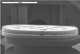
The stacked filters were found to remain bonded after cryogenic thermal cycling. Furthermore, the size of the passband is larger for the stacked filters; a representative transmittance curve is presented below:
