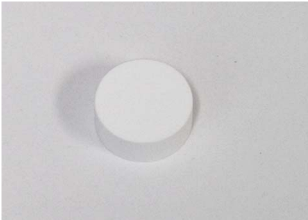
Fig.1.b: 99% white Spectralon test diffuser
