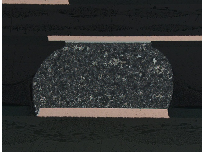
Figure 36. Mixed solder: PBGA postflight, ground unit.
