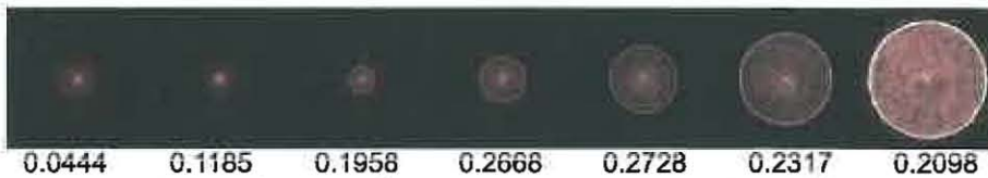
Figure 10 – The retrieved PSFs. The NRMSE between the retrieved and measured PSF is also reported for each plane.
