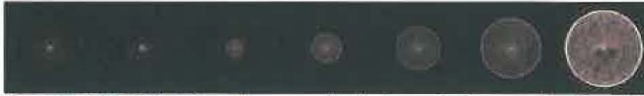
Figure 8 – The measured PSFs. The left-most image was collected at approximately paraxial best focus. The right-most image was collected at approximately marginal best focus. The distance between each data plane is 5 mm.
