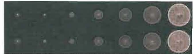
Figure 7 - The measured (top) and retrieved (bottom) PSFs. The left-most image was collected at approximately parallel best focus. The right-most image was collected at approximately marginal best focus. The distance between each plane is 5 mm.
