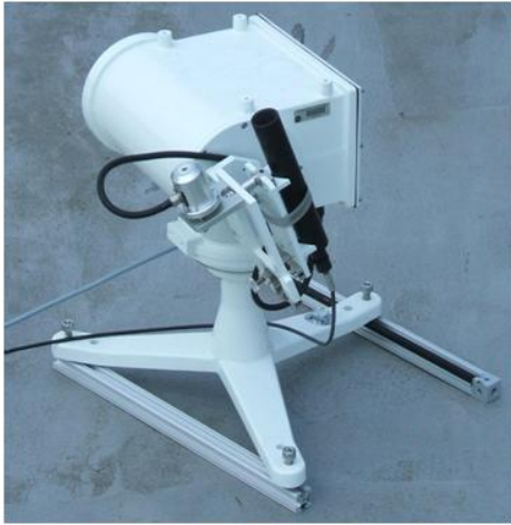
Figure 5. The telescope attached to the suntracker focuses an image of the sun on the end of a 52 fiber bundle used to conduct light down to the instrument in the lab.
