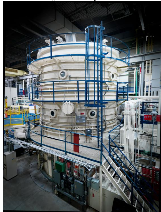
Figure 4: The 20-foot chamber at the Johnson Space Center used for a series of integrated life support testing in 1996 and 1997 3,4
