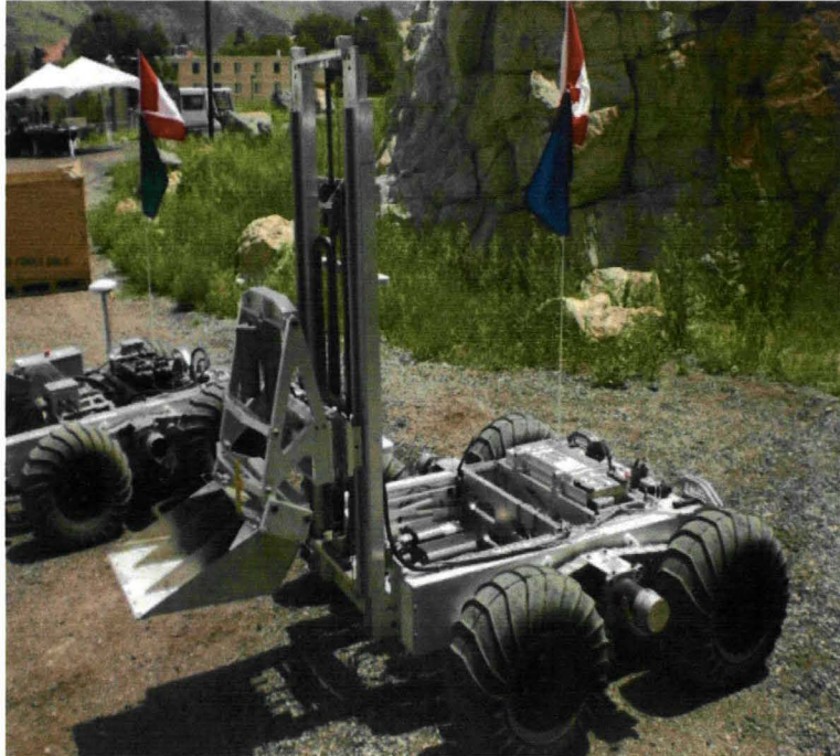
Load, Haul, Dump Excavator
